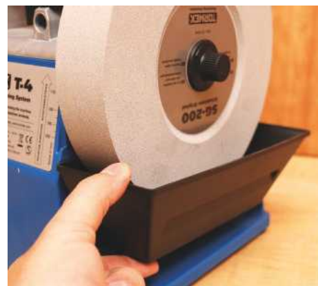
▲ The water trough clips easily onto the body
